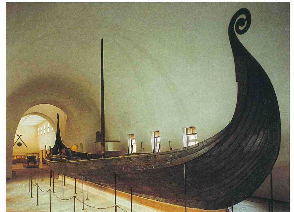
Figure 1-15 Almost 25 metres long, 5 metres wide, and 2 metres deep, this typical ninth-century Viking ship could carry a crew of thirty-two and sail into water just over a metre deep. In 1893, a small crew sailed a replica of a Viking ship across the Atlantic Ocean.
